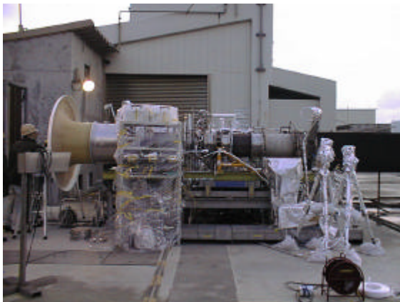
Figure 2: Experimental Turbo-Ramjet Engine at Noshiro Testing Center
